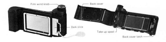
With the back cover latch pulled out, close and lock the back cover by pushing in the latch while pressing the back cover toward the holder. While observing the window which should indicate the picture size to be photographed, turn the film wind knob clockwise until figure 1 (printed on the backing paper) appears in the window.
