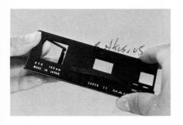
indicator window to 250, a bright frame for the 250mm lens can be observed in the finder. Determine the field of view center based on this frame.
